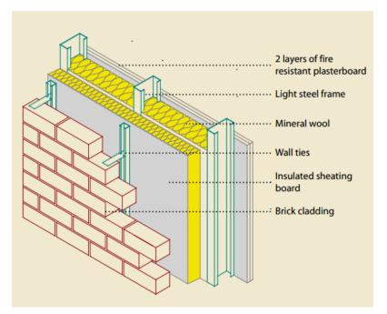
Figure 1 – Typical Steel Frame Construction <sup>1</sup>
