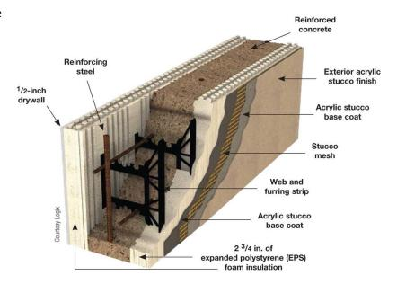
Figure 3 – Typical ICF Construction<sup>2</sup>
