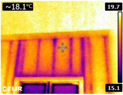
Figure 2 – Thermographic Image of a Steel Frame Construction Halifax, March 23, 2017
